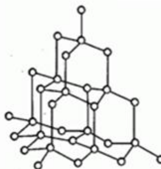
Fig.2 The structure of diamond showing four covalent bonds to each carbon atom.
